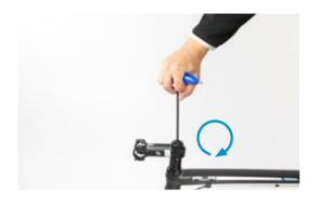
Satisfied? Secure the allen bolt properly, without over-tightening it! You need to make sure there's no play in the headset. Don't over-torque the bolt, as this will prevent the headset bearings from moving smoothly. This is detrimental to your bike's handling!
