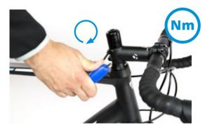
If you're satisfied with the set-up, then do up the bolts on the side of the stem. Once again, use a torque wrench if you have one.
