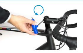
Want to adjust the height of your handlebars? Then you'll have to remove the stem first. Start by undoing the allen bolts on the side of the stem. The bolts don't have to be fully removed, just properly undone.
