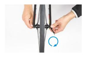
Now turn the securing bolt clockwise on the quick release (it should be on the drive-side of the bike). Hold the lever on the other side in the "open" position, preventing it from turning with the bolt.
