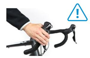
Apply the rear brake. Is there enough cable tension or oil pressure, and does the lever stay clear of the handlebars? Great! Check the front brake in the same way.
