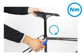
We've placed assembly grease or carbon paste in the seat tube, so you can just slide the seat post into the tube. Hold the saddle in your hand and align the saddle with the bike's top tube. The other hand can then tighten the allen bolt. Use a torque wrench if you have a carbon frame!
