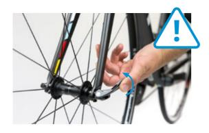
Once the securing bolt has been properly fastened, you can close the quick release lever. The lever in the "Closed" position should be parallel to the front fork.
