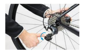
By carefully pushing down on the end of the derailleur cage, the frame should drop onto the rear wheel.
