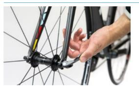
Check whether your wheels are secure, so check the through axles or quick releases.
