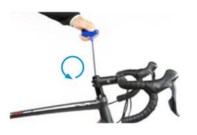
Now undo the allen bolt at the top of the stem (top-cap) all the way and remove it.
